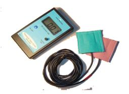
Power supply: 9 V battery. 10mA max
